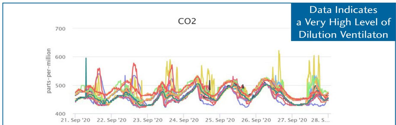
Figure 1 - Room Air was Tracking Ambient Outside Air (OA) of 450 ppm
