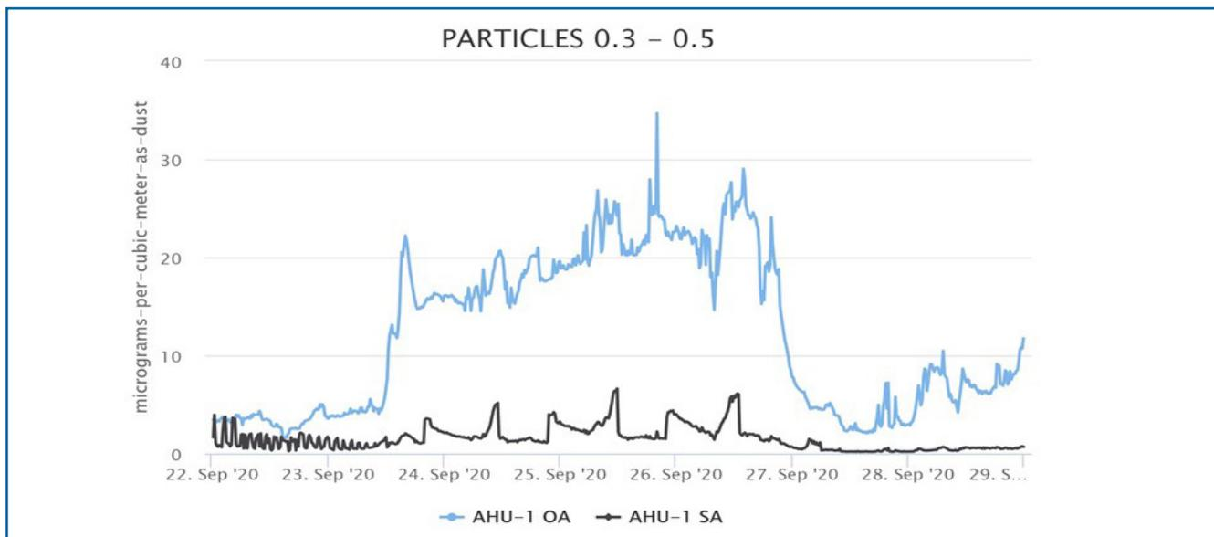
Figure 4 - Particles 0.3–0.5µm at the Air Handling Unit Level
