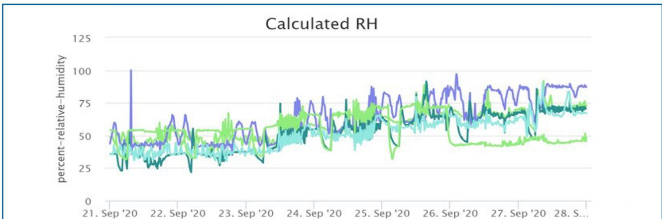
Figure 6 - Data Shows Average RH at Each Air Handling Unit
